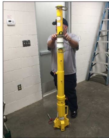
Figure 8. Fall arrest anchor post (left) and post ground anchors (right).
